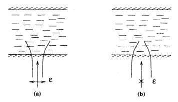
Figure 1: Effect of thermal indexing on beam width.
