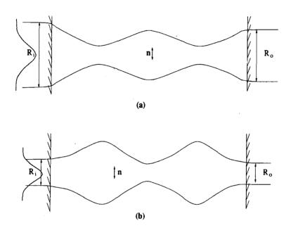
Figure 6: (a) The modulation of the beam width when the intensity  $I < I_m$ . The beam initially converges and repeatedly undergoes divergence and convergence. (b) The beam width initially increases on entrance when the intensity is  $I > I_m$ . On propagation, the beam width periodically increases and decreases.
