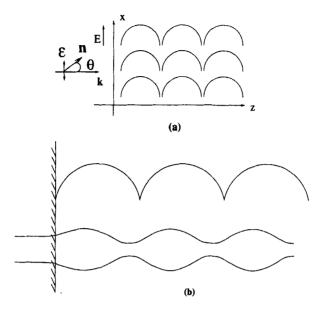
Figure 8: (a) The flexoelectric lattice in the presence of a static electric field. The periodicity is along the z direction perpendicular to the electric field(x axis). The laser beam is propagating along the periodicity axis. (b) The periodic variation of the beam width due to inhomogeneous periodic nonlinearity induced by thermal indexing.
