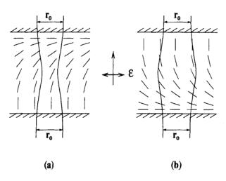
Figure 7: A hybrid aligned nematic. The beam transformations are shown in the figure. The beam width at entrance is the same at the exit and entrance points. (a) Laser incident on the homeotropically aligned surface. (b) Laser incident on the homogeneously aligned surface.
