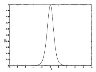
Figure 2: A typical soliton solution(5) of the generalised nonlinear Schrödinger equation (equation (4)) resulting due to the process of laser suppression of the director fluctuations alone. X is the transverse coordinate scaled with respect to the wavevector,  $X = x * k_o$  and  $\psi(X)$  is the amplitude of the laser field.
