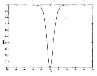
Figure 3: A typical dark soliton solution(8) of the nonlinear Schrödinger equation resulting due to 'thermal indexing' alone. X is the transverse coordinate scaled with respect to the wavevector,  $X = x * k_0$  and  $\psi(X)$  is the amplitude of the laser field.
