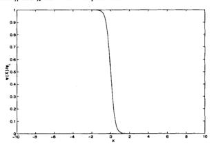
Figure 4: A kink soliton solution of the nonlinear Schrödinger equation (equation (11)). The parameters in the equation are as follows:  $\psi_L = 60.945$ ,  $\nu = 20.3$ ,  $\zeta = 4.5$  and  $\gamma = 0.01$ . X is the transverse coordinate scaled with respect to the wavevector,  $X = x * k_0$  and  $\psi(X)$  is the amplitude of the laser field.
